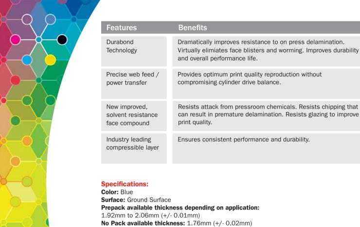
No Pack available thickness: 1.76mm (+/- 0.02mm Metal Backing: 0.20mm Stainless Steel Backing Face Compound: Solvent Resistant Rubber Blend
