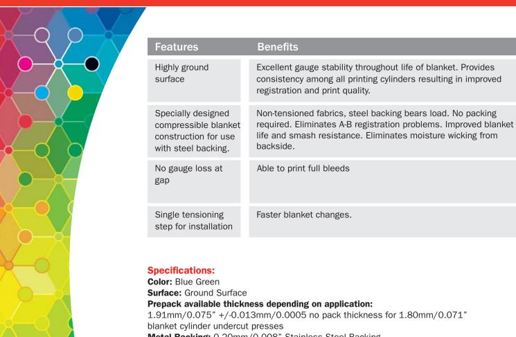
Metal Backing: 0.20mm/0.008" Stainless Steel Backing
