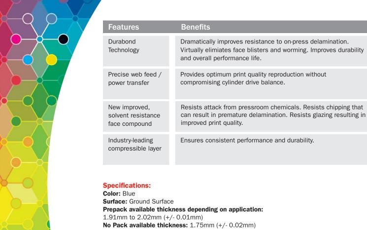
No Pack available thickness: 1.75mm (+/- 0.02m Metal Backing: 0.20mm Stainless Steel Backing Face Compound: Solvent Resistant Rubber Blend
